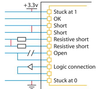
Find a wide range of faults using XJDeveloper's connection test
